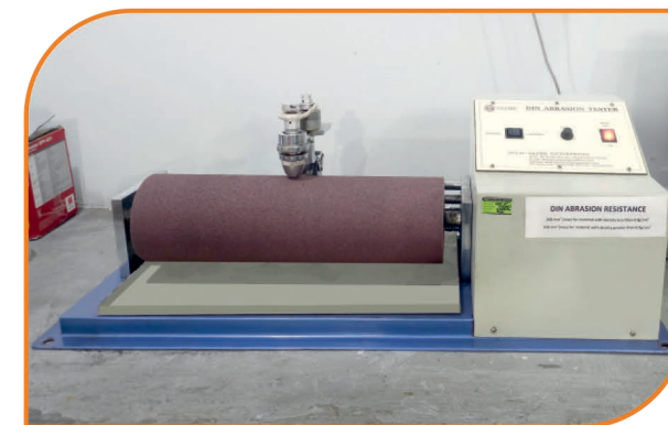
SOLE ABRASION RESISTANCE TEST
